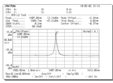
Channel on Extended L-Band (1607.08 nm)<sup>1</sup>
