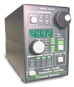
Power Supply: 115 / 230 VAC 60 / 50 Hz Temperature Control Output Current: up to  $\pm 5$  A Temperature Stability: 0.001°C (10 k $\Omega$  thermistor at 25°C) over one hour Stability across ambient: 0.001°C (10 k $\Omega$  thermistor at 25°C) over an hour ---- Ideal for scanning app
