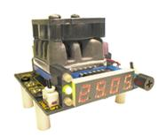
The **WTC3293-14001** is a mini-instrument temperature controller with a temperature (not resistance) display and onboard adjustments.
