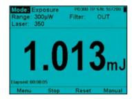
Exposure measurement (energy summing) with photodiode sensor.
