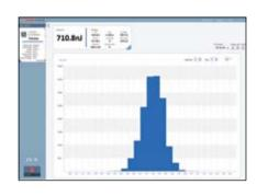
The built-in USB and RS232 interfaces and StarLab PC software allow display and processing of data either in real time or from previously stored data. Results are displayed graphically on a PC. To support PC interfacing, LabVIEW drivers, a COM Object Interface and demo source code are provided.
