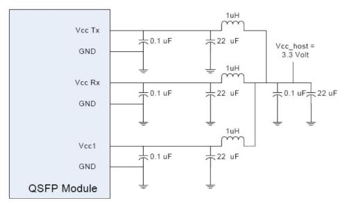
Figure 2.QSFP voltage supply and filtering scheme
