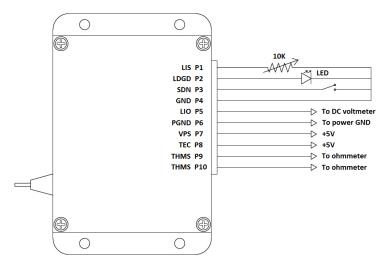
Figure 2. Stand-alone Application Schematic for PPM-003C
