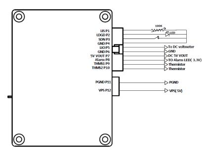
Figure 2. Stand-alone Application Schematic for PPM-010C
