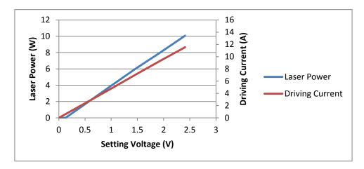
Figure 3. Laser Power & Driving Current under Different Voltage Settings
