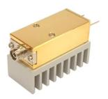
**Passive Heatsinking Option:** Custom heatsinking can be easily applied to the YCH-H003 PPC to generate higher power output, and higher performance. Heatsink size will depend on the application's operating conditions and power requirements. The below summarizes the performance of the YCH-H003 PPC with 50 x 24 x 16 mm aluminum heatsink. An efficiency of ~26% with 10W input is achieved:
