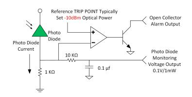
All alarms are Open Collector topology, with Active Low for Normal operations and during Alarm condition the open collector will Pull to High logic levels. Reverse polarity alarm is also available upon request, such as under normal conditions the Open collector will be High and vice versa under fault conditions.
