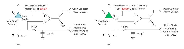
All alarms are Open Collector topology, with Active Low for Normal operations and during Alarm condition the open collector will Pull to High logic levels. Reverse polarity alarm is also available upon request, such as under normal conditions the Open collector will be High and vice versa under fault conditions.
